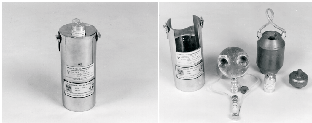
Fig. 16.3 Alumina column chromatography generator for ^{99m}\text{Tc} and components.
